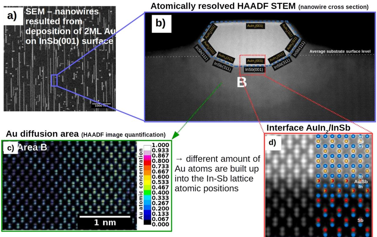
**Figure:** Nanowires on InSb(001) substrate resulted from deposition of 2ML of Au at 330C. a) SEM image showing the wires, b-d) Atomically resolved HAADF STEM showing detailed atomic structure with chemical sensitivity (Au atomic columns appears brighter than In-Sb atomic columns).
