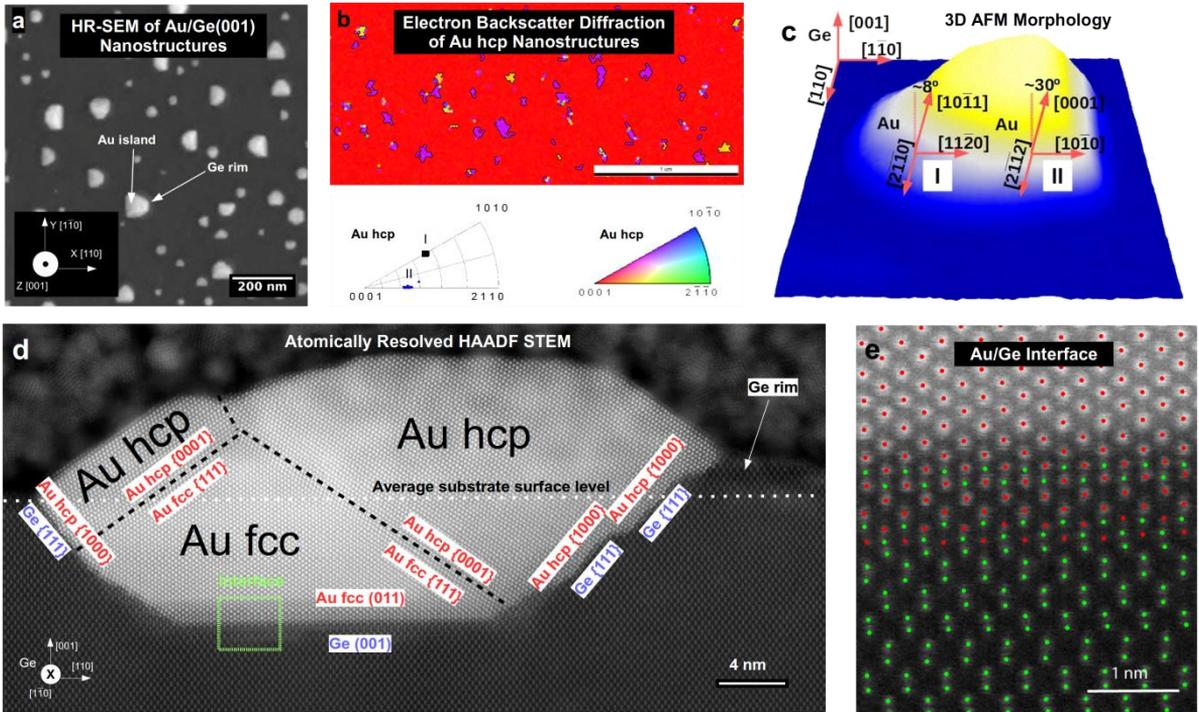
**Figure 1:** Self-assembled Au hcp nanostructures on Ge(001) surface. a) HR-SEM, b) EBSD IPF, c) 3D AFM, d) Atomically resolved HAADF STEM, e) Au/Ge interface (Au atoms – red, Ge atoms - green)
