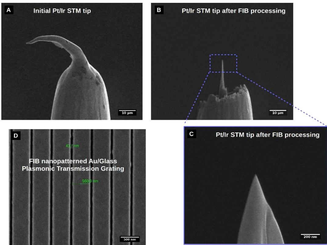
**Figure 1: FIB sharpening of Pt/Ir STM tip a)-c), FIB nanopatterning of Au/Glass Plasmonic Transmission Grating**
