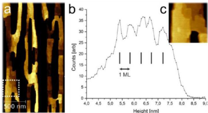
**Figure 1:** TM-AFM image of 0.25 ML coverage of 6P on TiO<sub>2</sub>(110): a) View on the top of the nanoneedles. b) Height histogram of nanoneedles. c) Monolayer terraces of the lying molecules imaged on top of the nanoneedles.
