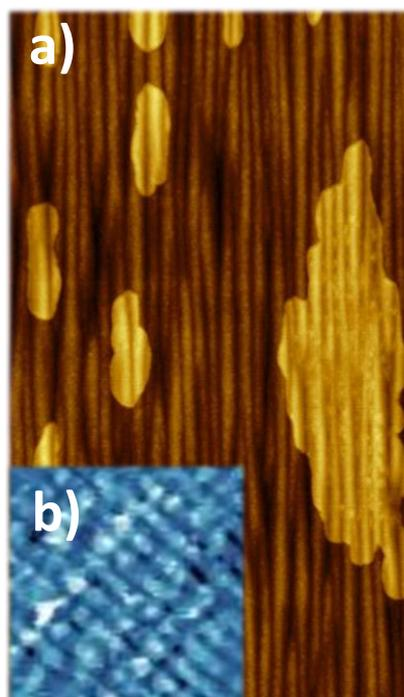
**Figure 2:** a) NC-AFM image of 0.5 ML coverage of 6P on rippled TiO<sub>2</sub>(110). b) View on the top of the islands with molecular resolution.
